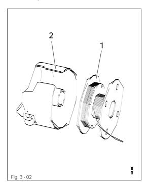
Insert bobbin 1 in the bobbin case 2 as shown in Fig. 3 - 02.
